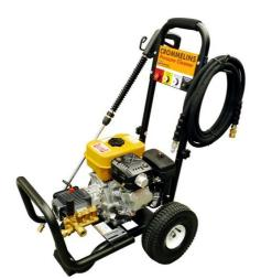
Extremely popular, assembled and tested in Australia, the 2700psi CPV2700X21 is powered by a 7.0hp Subaru engine, providing constant rpm and allowing a continuous and reliable 11.4L flow of water pressure per minute.
